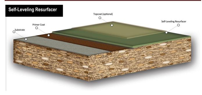
Epoxy Mortar Flooring System is a self-leveling, high strength concrete resurfacing material. It is used for environments requiring a highly smooth industrial grade floor or when a concrete floor has sustained damage requiring a 1/16" to 1/8" surface restoration.
